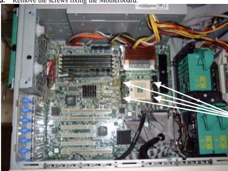
Remove the screws fixing the Motherboard.
